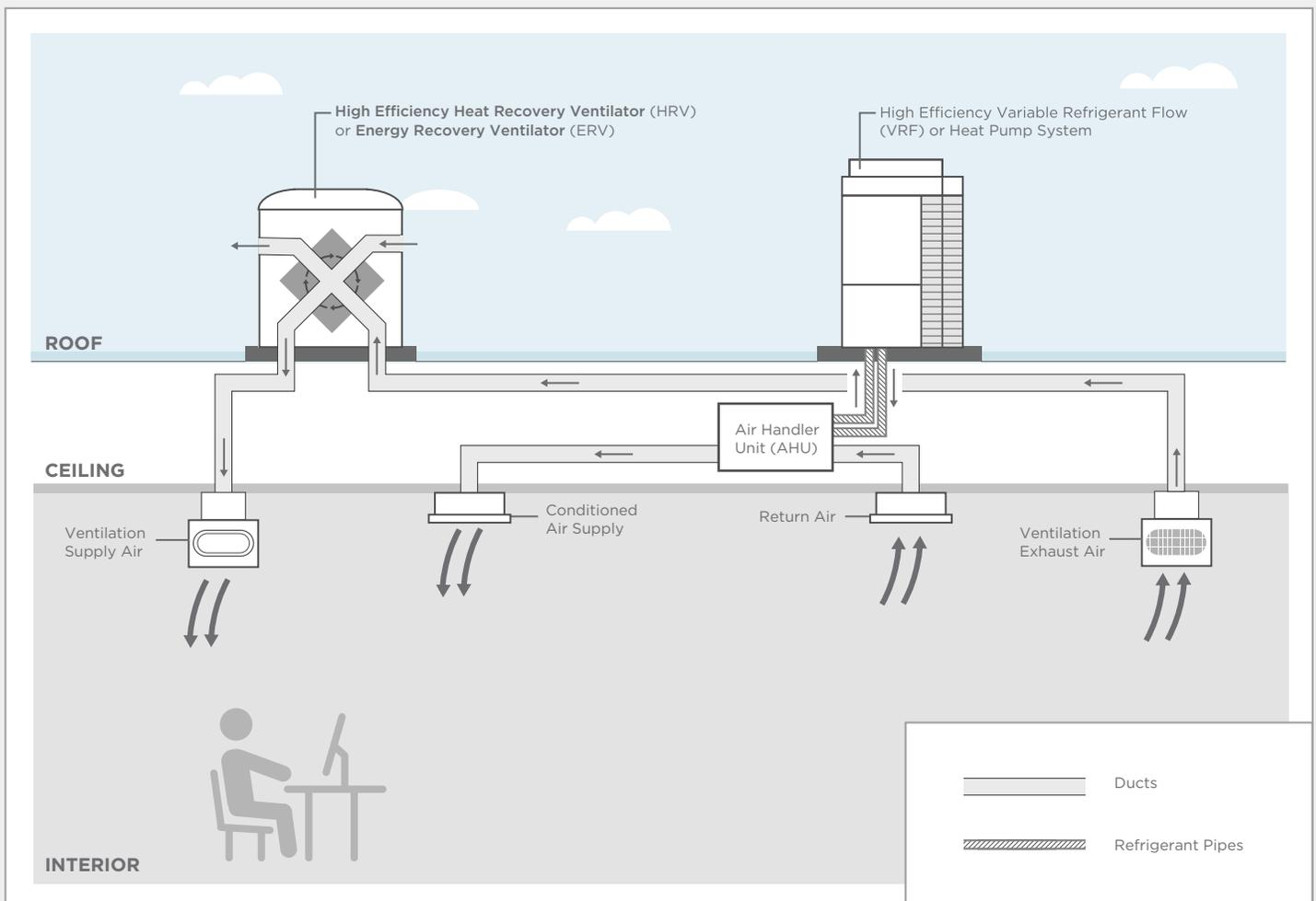
*Note: This drawing is for quick-reference only and does not represent the sizing or depth of the system or frame for all manufacturers' products. Please check with manufacturer for exact measurements and specifications.*
